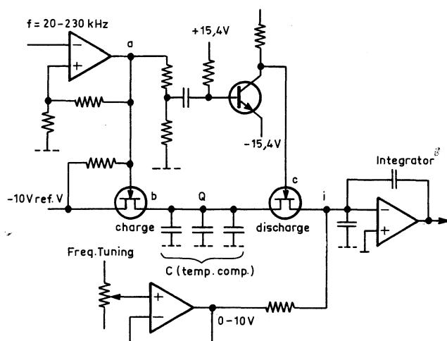
The input frequency  $f$  is applied to a Voltage Comparator which produces the square wave signal  $a$ . When this signal is at 0V the capacitors  $C$  are being charged to the ref. voltage of -10V.
