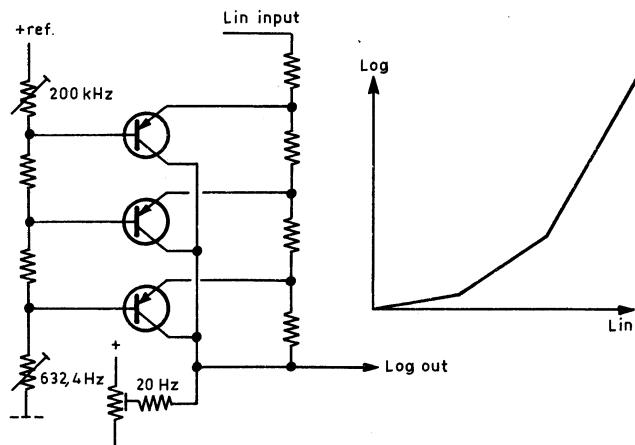
In connection with the Lin./Log Converter, a temperature compensating circuit is used.
